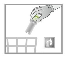
Dispose of the HPKV cartridge in any normal waste bin.
